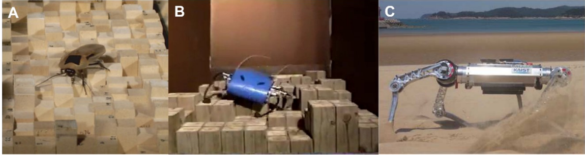
Figure 1-6: Animals and robots maintain the stability when traversing rough terrains. (A) A cockroach traverses rough terrain with only mechanical feedback. (B) A RHex robot traverses rough terrain without sensory feedback. (C) A Raibo robot traverse deformable terrain with sense-based modulations. Image courtesy of (B) Agile Systems Lab at Georgia Tech on YouTube. (A, C) Adapted from [74,77].
