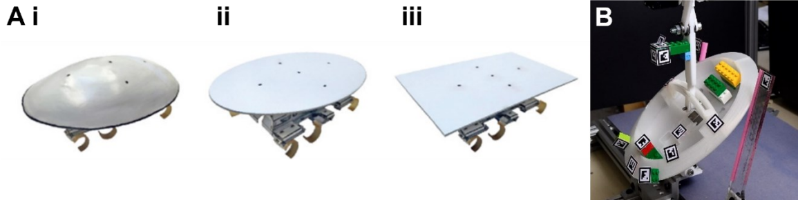
Figure 1-12: Robophysical models. (A) Legged robots with (i) ellipsoid slice, (ii) flat oval, and (iii) Flat rectangle shells. (B) Simplest robophysical model. Adapted from [31,36].
