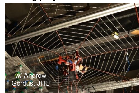
Robotic modeling of web spider sensing prey via web vibrations
