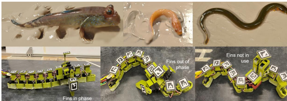
Fig. 12. Fish robot for studying amphibious fishes crawling on mud.
