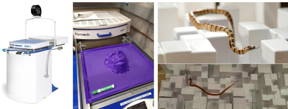
Fig. 5. Thermal former for making custom complex shapes, such as uneven terrain for studying snake locomotion in complex 3-D terrains.
