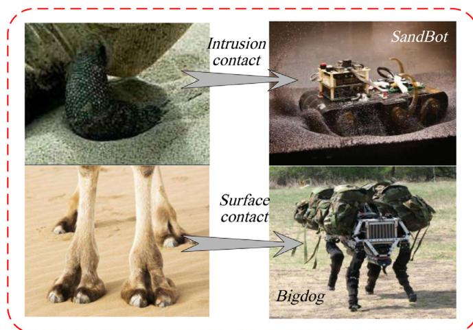
**Fig. 1.** Diagram of difference between the intrusion contact of lizard and surface contact of camel with sand particles, both types of interaction mechanisms have been implemented in legged robots, such as hexapod SandBot [5] and quadruped robots Bigdog [3]
