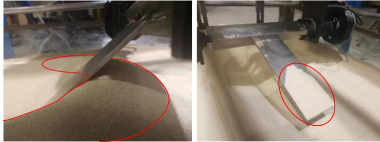
Fig. 8. Accumulated rising parts at two different obliquities.
