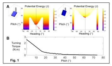
model predicted that the attractive torque (potential energy gradient along the heading direction) towards the obstacle decreased as body pitch increased (Fig. 1B). This meant that, if the robot pitches up more, it needs less torque from leg adjustment to turn its body to escape the obstacle.
